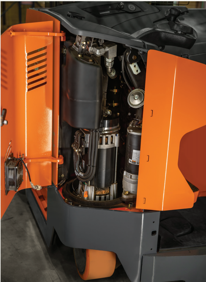
AC Drive and Lift Motor
